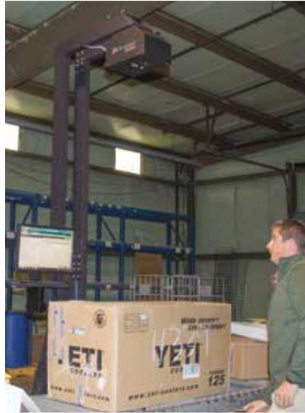
Installed over their pre-existing conveyor line, iDimension 300 streamlines dimensions, package images and weight data with third-party postal software to ensure the most cost-effective shipping.
